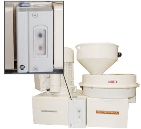
Motor protection on the back of the mill
